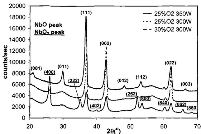
FIG. 1. XRD phase scans of niobium oxide films deposited under different oxygen concentration and sputtering powers. Samples were measured after 800 °C 5 min anneal in Ar.
