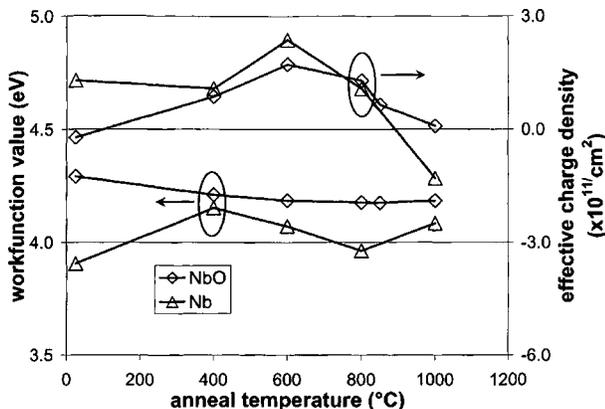
FIG. 3. Work functions and effective charge density change for NbO and Nb over a series of anneals.
