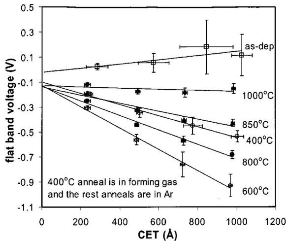
FIG. 2.  $V_{fb}$  vs CET for NbO measured over a series of anneals. Gate dielectric is  $\text{SiO}_2$  with different thicknesses, error bar in the figure is the cross-wafer variation. Work function value could be extracted from y intercepts.
