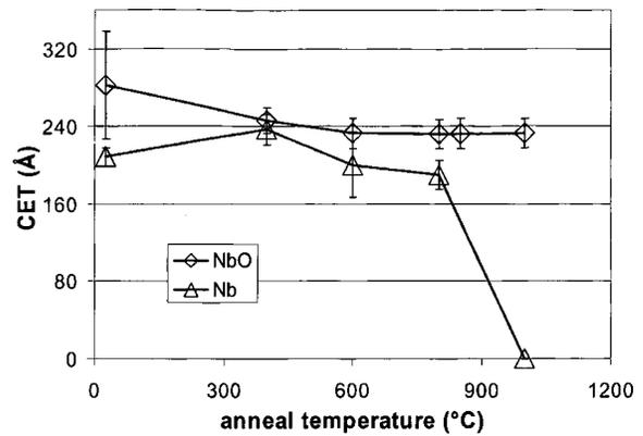
FIG. 4. CET stability of Nb and NbO on  $\text{SiO}_2$ .
